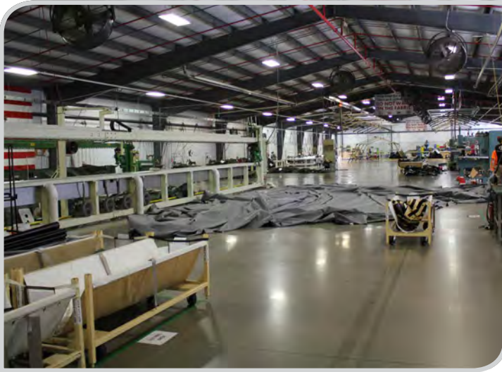
WIP CART ENABLED PRODUCT FLOW BY-PASSES PERMANENT FIXTURES
